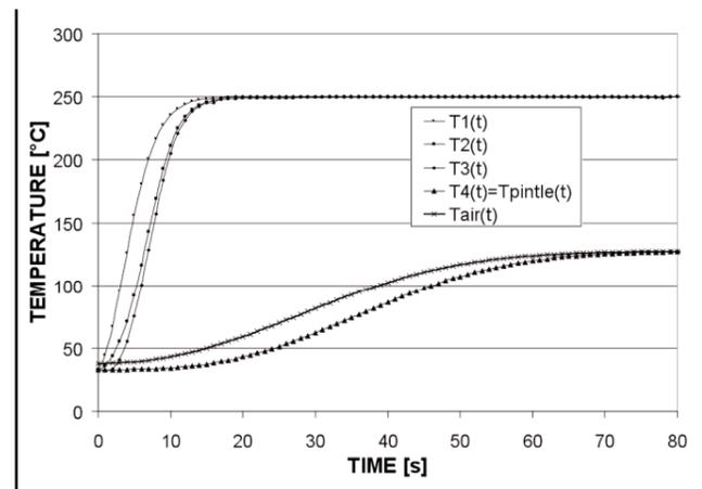
Thus, considering the flow conditions and the heat transfer phenomena for each element, the temperature variation in time was evaluated. Fig. 6 and 7 represent temperature variation found when the EGR gas flow reaches the valve at 250°C and 500°C respectively.
